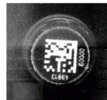
Gelaserter Code (im Original 2,4x2,4mm)
