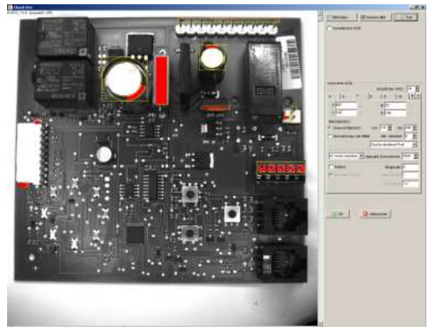
Layout check of circuit boards
