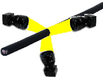
Example camera positions cable surface inspection
